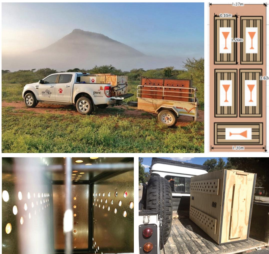
**Image 2.** Wooden International Air Transport Association (IATA) specification crates made by A.W. Gilson and used by EWT for safe transportation of cheetah in South Africa.
